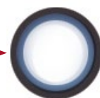
Cell filled and free of air bubbles
