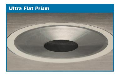
The flat open sample area has no corners to trap even sticky materials and is resistant to almost all solvents including Acetone, Toluene and similar organics. Choose H option for HFl and HCl acids.
