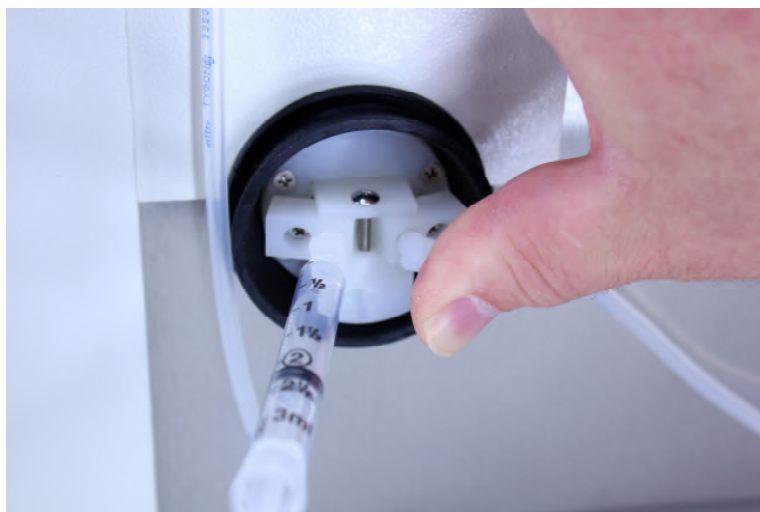
Figure 5.4 Checking the Filling Nozzles for Air Tightness
