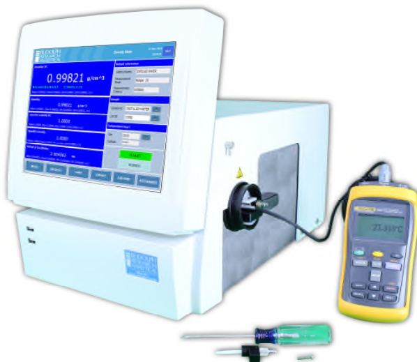
Figure 9.12 – Temperature Verification with a certified Fluke-Hart Thermometer
