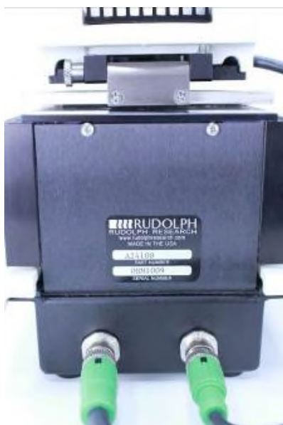
Figure 5.6 – OBM to Display Base (on right) and Optics Box to Presser cable (on left)
