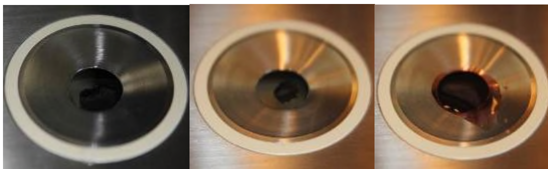
Figure 7.5 – Sample Clean Prism Sample not correctly applied Sample Correctly applied
